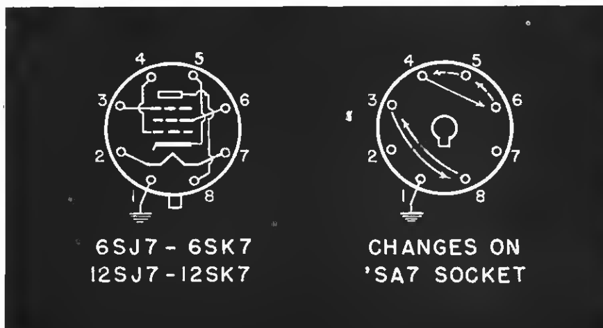
Fig. 1—Socket wiring changes to replace 12SA7 with 12SJ7 or 12SK7. The change reduces sensitivity but set will function for local station reception.
